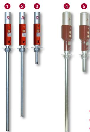
Eurolube 5:1 pumps are designed to dispense lubricating oils and similar products up to SAE 140 in piped systems. Models B15780-2 are recommended for simultaneous use up to 3 outlets. Models 15770-1 are recommended if more than 3 outlets are in use simultaneously. The pumps can deliver motor oils, gear oils, cutting oils, hydraulic oils, machine coolants, automatic transmission fluids and a wide range of petroleum-based fluids from pails, drums, tanks and IBC containers.
