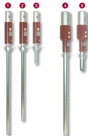
Eurolube 3:1 pumps are designed to dispense lubricating oils and similar products up to SAE 90 in piped systems. Models A13760-2 are recommended for simultaneous use up to 3 outlets. Models 13765-6 are recommended if more than 3 outlets are in use simultaneously. The pumps can deliver motor oils, gear oils, cutting oils, hydraulic oils, machine coolants, automatic transmission fluids and a wide range of petroleum-based fluids from pails, drums, tanks and IBC containers.
